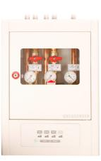
02-01, for shutting off individual stations or functional areas of the central gas supply system. The Ventus is protected against unauthorized opening by an electronically monitored door. It is suitable for under plaster mounting, mounting in dry walls or surface mounting. The rear part is made of galvanized sheet steel. The window allows a quick reading of the manometer and valve positions in closed condition.
