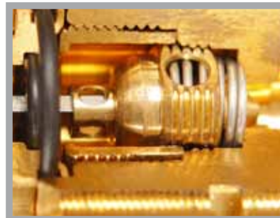
After approx. 3-4 rotations, the rear part of the terminal unit is sealed gas-tight. Maintenance work, for example the replacement of the sealing cartridge or replacement of the entire front part, can be easily performed under operating pressure.
